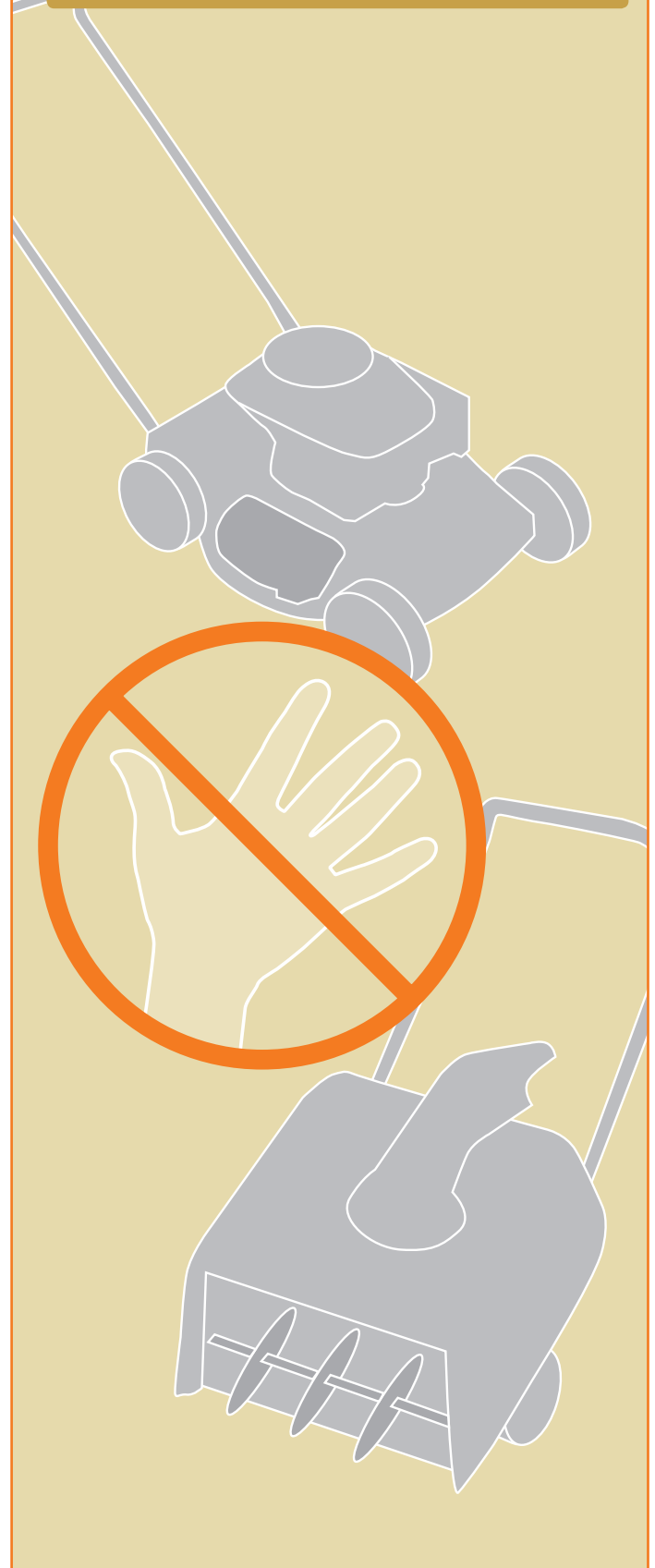
Figure 1. After the machine is turned off and unplugged, any obstruction should be removed with a tool and not the hand or fingers.
